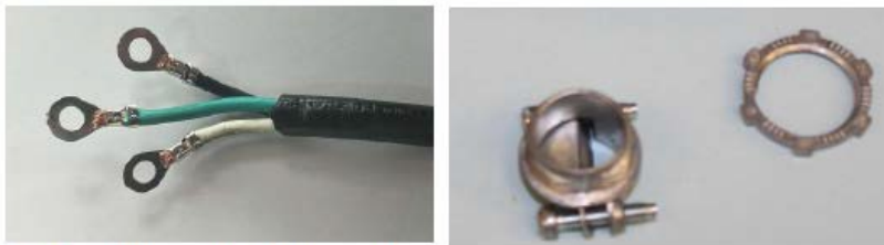
Figure 11: Installing cable fitting to heater
