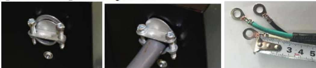
Figure 11: Installing cable fitting to heater
